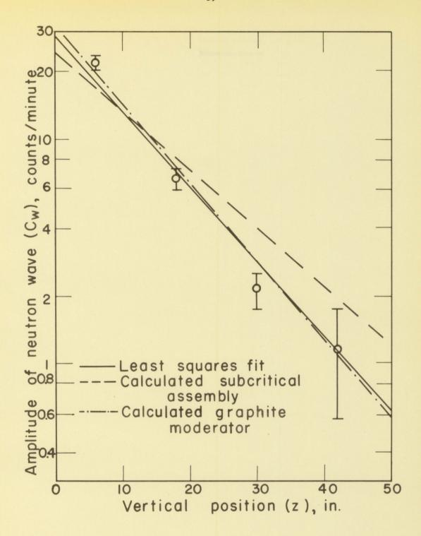
Fig. 10. Amplitude attenuation with vertical position for 380 r.p.m.
