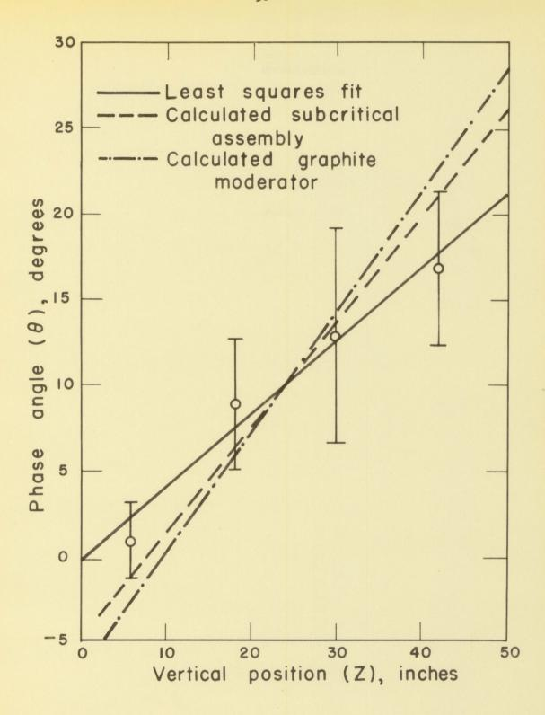
Fig. 7. Phase angle variation with vertical position for 380 r.p.m.
