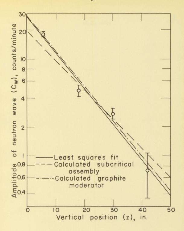
Fig. 9. Amplitude attenuation with vertical position for 190 r.p.m.
