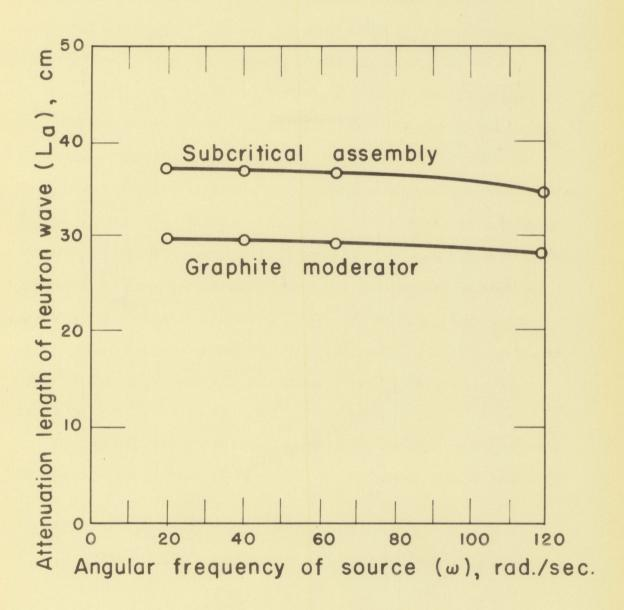
Fig. 6. Calculated attenuation length of the neutron wave
