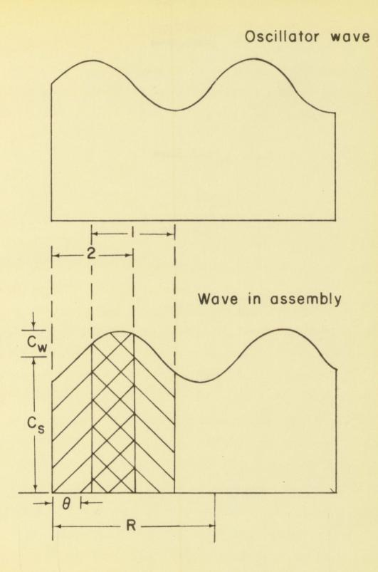
Fig. 4. Phase shift of neutron wave in assembly
