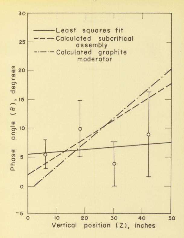
Fig. 8. Phase angle variation with vertical position for 190 r.p.m.
