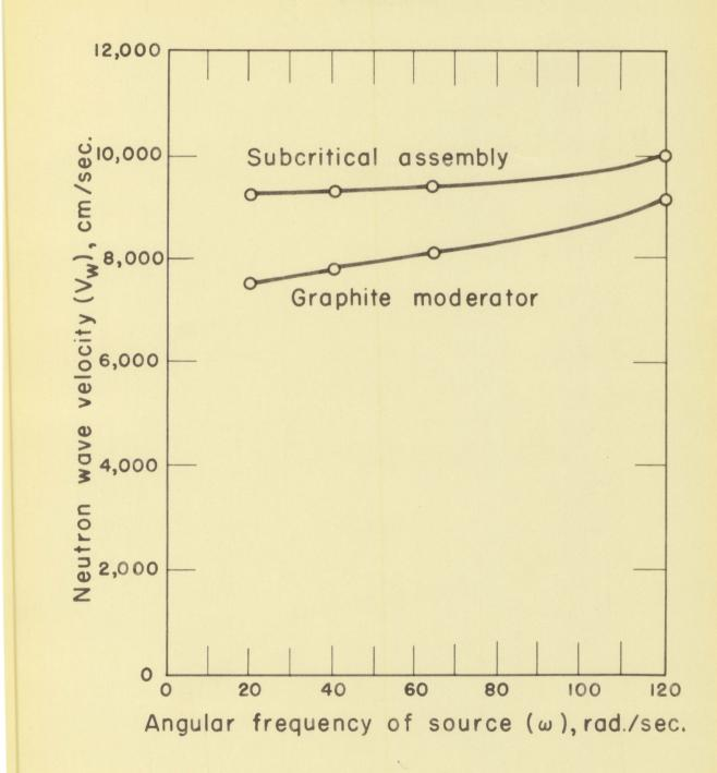
Fig. 5. Calculated wave velocity of the neutron wave
