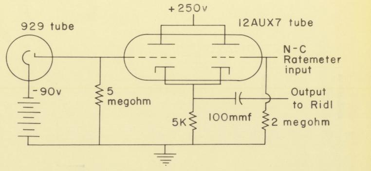
Fig. 3. Circuit diagram of electronic switch
