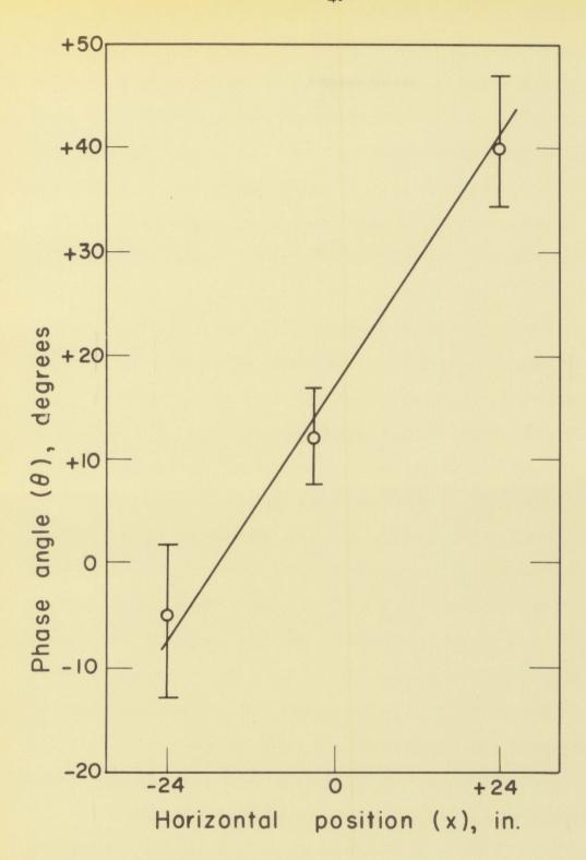
Fig. 11. Phase angle shift with horizontal position at the 24-in. level
